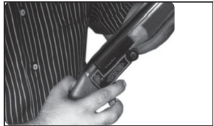
Push the safety button for safety mode. When the shotgun was in this mode, you can not see "red alert" colour on safety button. Important : Please keep the shotgun in safety mode everytime while you are not shooting.
