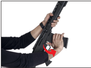
1- Press hook, remove the magazine.
