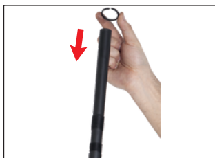
4- Put big washer on the barrel.
