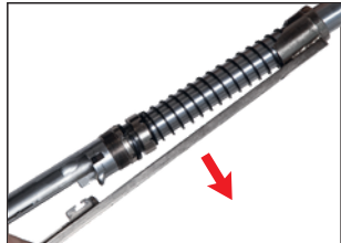
12- Remove bolt, and bolt carrier.
