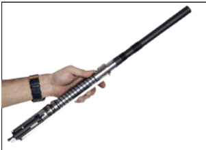
11- Remove bolt barrel assembly.
