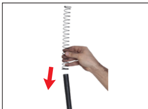
6- Put barrel and bolt carrier spring.
