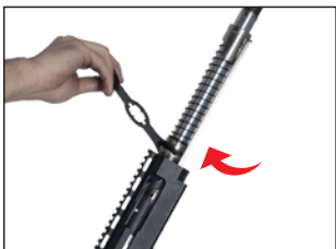
11- Fixed both of nuts tightly on the barrel.
