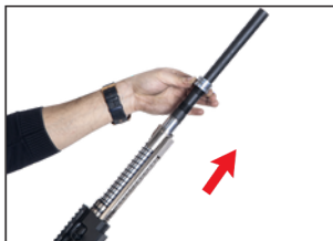
7- Now remove piston by pulling it upside.
