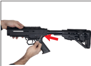
13- Remove upper lower by removing pins.
