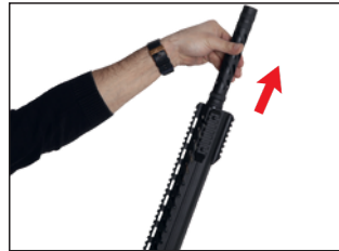
2- Remove barrel shroud by moving it anticlockwise.
