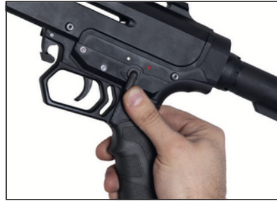
White dot, safety is on gun is ready to fire Red dot safety is off
