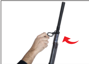
17- Gas chamber nut is fixed.
