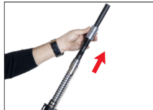
6- Remove gas chamber.
