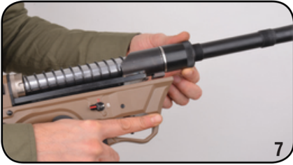
7. Remove the Gas Chamber by Turing it towards the Right side.
