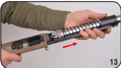
13. Remove the arm by pulling the mainspring inside the mechanism.
