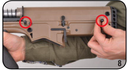
8. Pull out the locking pins from the lower receiver which can separate the upper and lower part.
