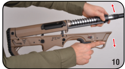
10. Separate the upper and lower body of the gun.
