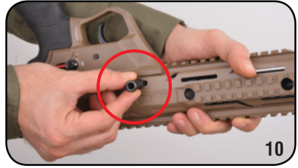
10. Place the charging latch from the right or left according to your choice.
