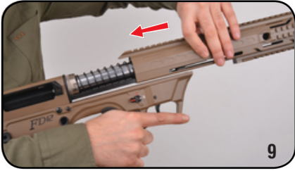
9. Connect the forend to the main body, Now put the Handguard centering cap.
